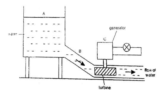
The water turns the blades in the turbine so that electricity is produced by the generator to light up the bulb.
